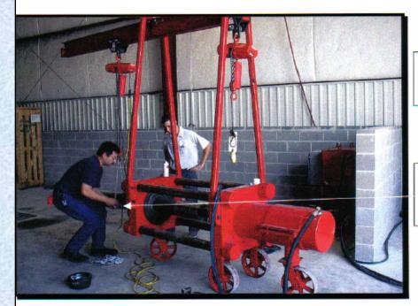
Swage Press swaging a 3 ½" Grade D Rotary Drilling Hose.
