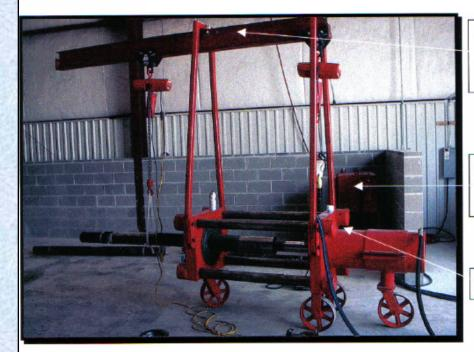
A-Frame and track with two ¼-ton electric hoist and trolleys.
